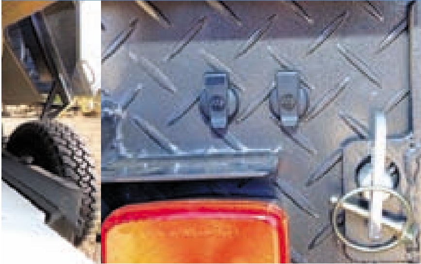
Simple and solid pretty much spells out the Trackabout range, with plentiful use of chequerplate protection and big pinned latches to match. There are four jerry can holders on the Safari and a 60L tank slung underneath – plenty of fuel and water for a dry country!
